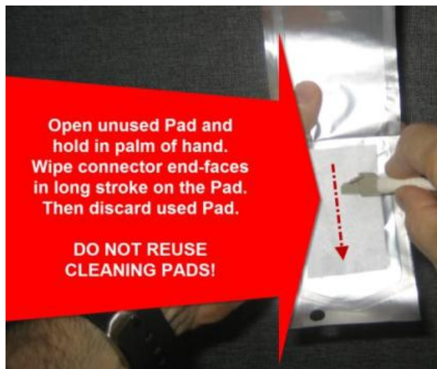
Figure 7. Clean Optical Plug with supplied Clean Wipes
