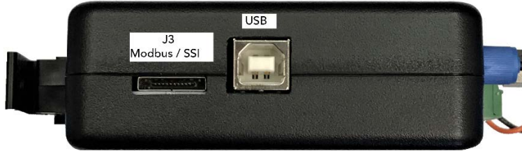
Figure 8. Location of SSI, RS485/Modbus RTU, and USB Connections
